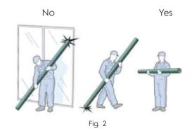
Avoid dragging pipes on the ground or against the sides and tailgate of the vehicle (Fig.2).
