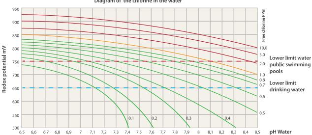
A simple method for ascertaining whether particular water is compatible with the use of PP pipes is to measure the oxidation-reduction potential using one of the many portable instruments available on the market, such as the one shown in the picture on the top. The potential must be less than 750 mV
